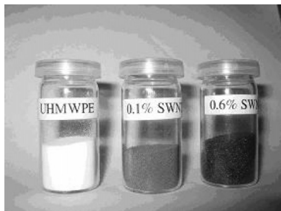
Figure 3. UHMWPE powders and SWNT–UHMWPE powders, with a weight percentage of 0.1% and 0.6% SWNTs prepared by the spraying technique.
